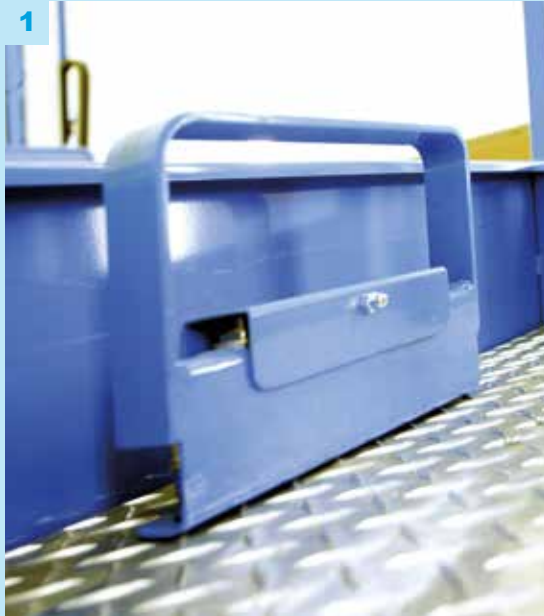
1 Foot pedal – as supplement to the three joysticks.
