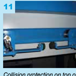
11 Collision protection on top of mast when more than one WALL-MAN® on same rail.
