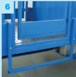
6 Access step to cage when needed.
