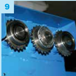
9 Chain drive – when upper rail is slippery.
